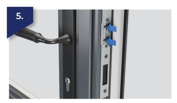
If you need to adjust the compression on door sashes, to ensure they open with minimal effort, but maintain a tight seal when closed. You can increase the contact pressure between the sash and frame as required by using the two machine screws indicated.
