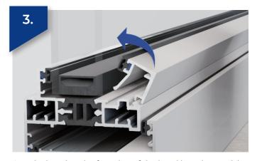
Start by locating the front leg of the bead into the receiving channel and rotate the bead until it 'clips' into place. Fit the top bead first to secure the unit. Continue by fitting the bottom bead and then the sides, being careful not to scratch the powder coated finish.
