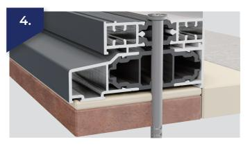
Fix the frame into the aperture using suitable frame fixings to suit construction material. Countersinking if required.
