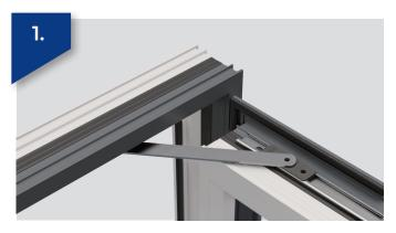
Locate datum bar against sash insert and screw the door restrictor into position on the sash using four 3.9mm x 16mm pan head self drilling screws.
