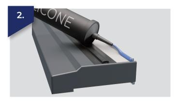
A co-extruded gasket on the cill, seals between the frame and cill along its length. Also apply a bead of silicone sealant along the inner edge of the upstand.
