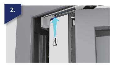
Once the sash is properly located it will be held firmly in place, allowing you to fix the hinge into position using 4.2 x 13mm pan head screws. Once complete, test for correct operation and repeat as required.
