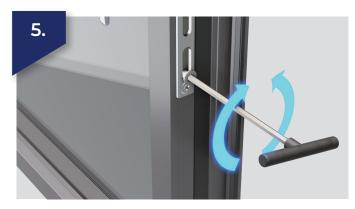
If you need to adjust the compression on window sashes, to ensure they open with minimal effort but maintains a tight seal when closed, adjust the locking pins on the espag lock using a 4mm allen key.
