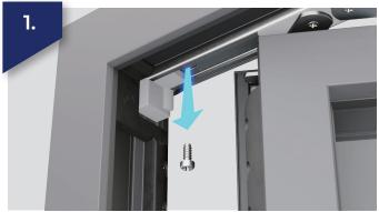
Remove sashes where possible (operational and dummy), to lighten the installation. Make sure you have a safe and protected surface to lay the sash once you've removed it. Start by unscrewing the sash.
