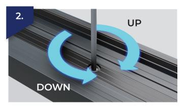
Using a 4mm Allen key, turn the grub screw clockwise to apply more pressure onto the packer, or counterclockwise to relieve pressure to adjust the weight distribution of the glass. This will allow you to bring the sashes into line and ensure a perfect finish to your Classic window installation.
