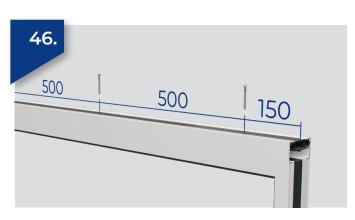
Fix frame extender 150mm from ends and max 500mm between centres using 4.3 x 55mm countersunk screws (or 4.3 x 35mm countersunk screws if the extender is flipped with the thermal break against the frame)
