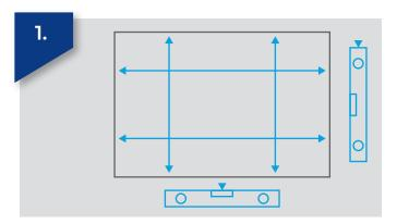
Ensure that all four sides of the aperture are plumb and square and identify any potential packing points. Please note our recommended fixing positions are into the outer wall and the frames are not fixed over an open cavity as this can compromise system performance.
