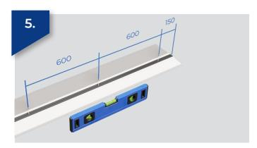
Fix 150mm from each end, and no more than 600mm between centres. Use a 1.8m level, laser level or suitable device to ensure the cill is level (+/-1mm per metre).
