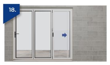
Next, fit the two vertical beads, being careful not to scratch the painted profile while fitting. Finally run your finger along the gasket edge to check they have seated correctly, adjusting if required.
