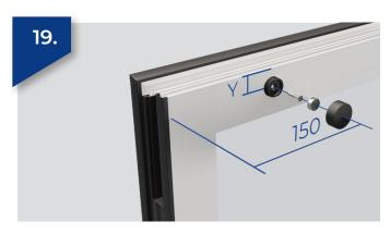
These magnet positions below are for regular width doors with double rollers. Fix 150mm in from edge of the sash. For vertical positioning please see point 22 below.
