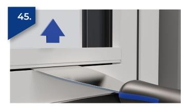
Push down on tool to disengage bead.
