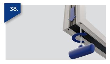
Fine adjustment of the corner joint can be done with a hand-held T25 Torx driver. Turning the cleat screw in a clockwise direction will draw the opposing profile toward you. It is important not to overtighten too much. We also advise gradually working on each cleat in turn to avoid stressing the corner cleat.
