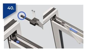
Slide & click the guide into position at the hinge end of the sash head.
