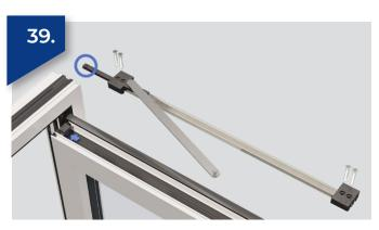
Locate datum bar against sash insert and screw the door restrictor into position on the sash using four 4.3 x 25mm countersunk screws.
