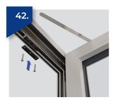
Mark & drill two 2.5mm pilot holes through the head track & fit the frame bracket and track location packer with two 3.9 x 30mm countersunk screws.
