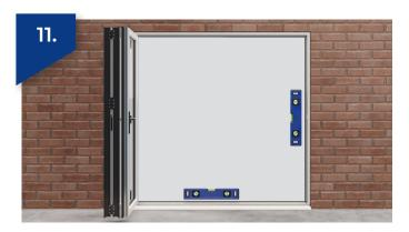
Finally check alignment of frame.
