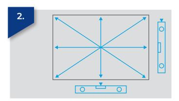
Ensure an adequate lintel or head linings are present, and are level and capable of supporting both the construction above and the bifold itself.
