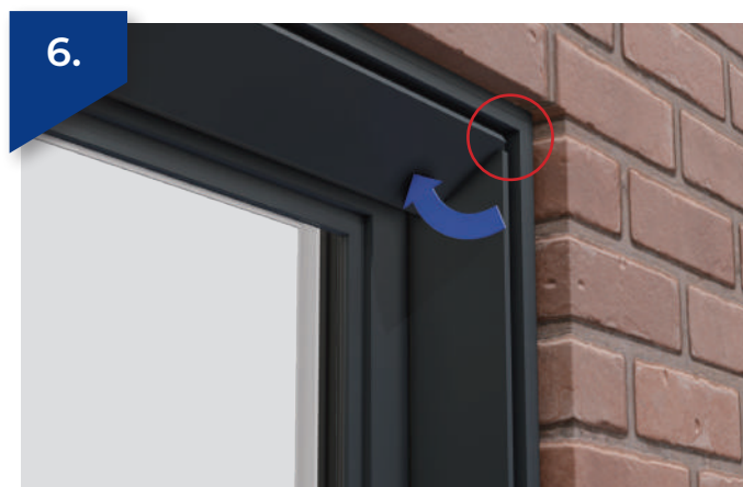
Fit jamb trim to head. Do not forget to fit the jamb trim corner shrouds top & bottom, handle side only (indicated above in red).
